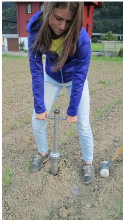
Figure 16: Pulling out the Humax drill containing soil
