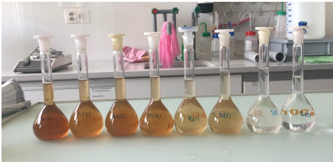
Fig. 6 Prepared solutions in the volumetric flasks after the process of saturating the soil with HCl.
