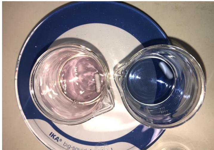
Fig. 5 Colour change of the Erio-T indicator from light pink to blue in the process of titrating
