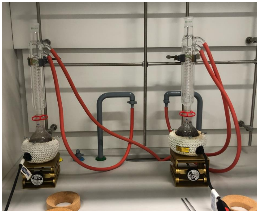
Fig. 8 Set up of the heating/cooling mechanism for the decomposition
