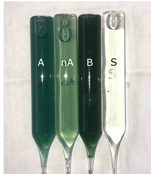
Fig. 21 Phosphate (PO 4 3- ) represented clearly in tubes A, nA and B.
