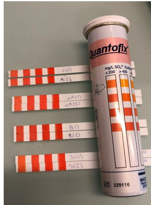
Fig. 19 Sulfate ( \text{SO}_4^{2-} ) lightly represented on strips S(1&2).
