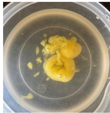
Figure 9: The big sphere burst in the alginate solution
