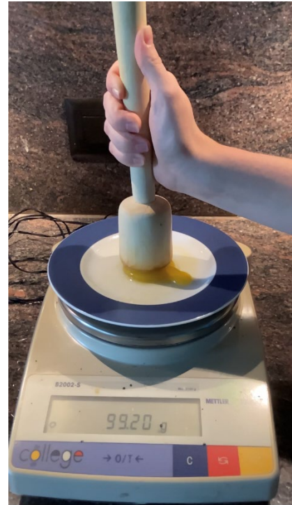
Figure 15 : Potato masher is used to press down on the sphere
