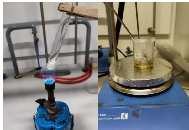
Figure 36: Mix of phthalic anhydride and ethanediol being heated over a Bunsen burner (left); the created yellowish hotmelt adhesive in a heated-up beaker, for it to remain in a liquid state (right).
