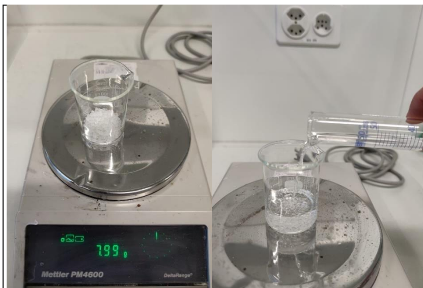
Figure 35: 7.99 g of polyvinyl acetate being weighed for the creation of all-purpose adhesive (left); 30 mL Ethyl acetate being poured into the polyvinyl acetate, before being heated up (right).
