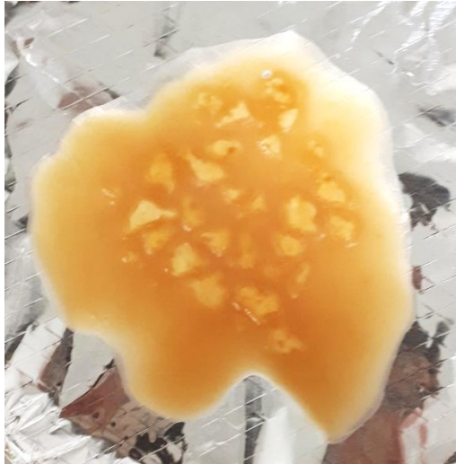
Figure 21 galalith with self-made casein on watch glass (left)
