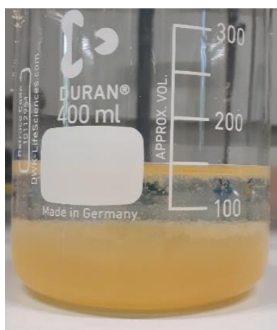
Figure 25 casein pieces after adding formaldehyde.
